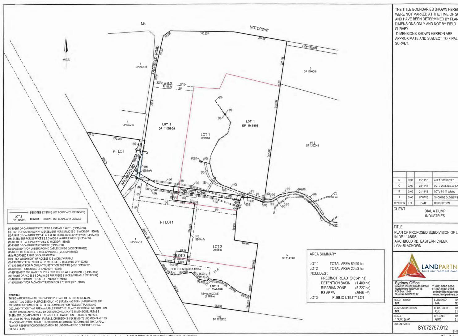
THE TITLE BOUNDARIES SHOWN HEREON WERE NOT MARKED AT THE TIME OF SURVEY AND HAVE BEEN DETERMINED BY PLAN DIMENSIONS ONLY AND NOT BY FIELD DIMENSIONS SHOWN HEREON ARE
